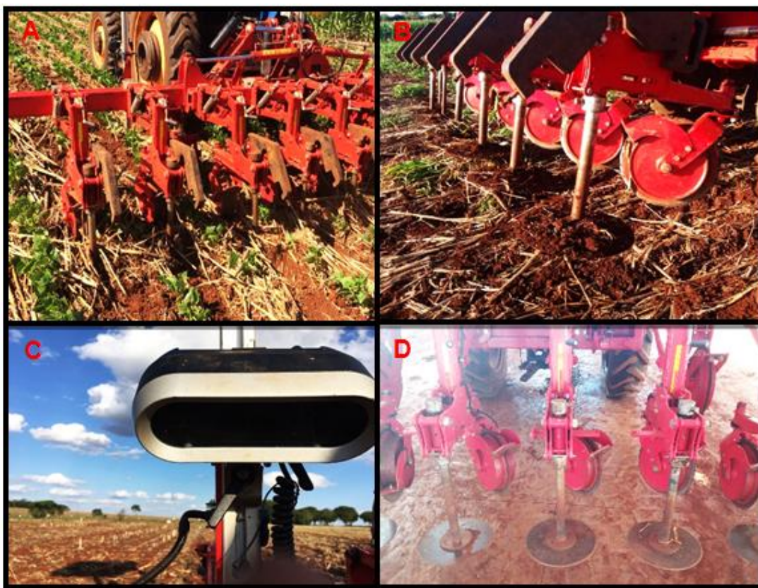
Fig. 1. Row hoe guided by video-camera adapted to be used in areas under direct sowing system. A: Automatized hoe in the bean crop; B: cut discs used to cut the straw; C: video-camera to detect the crop row; D: cut discs placed in the horizontal, with rotary axel, system used to cut the weeds
